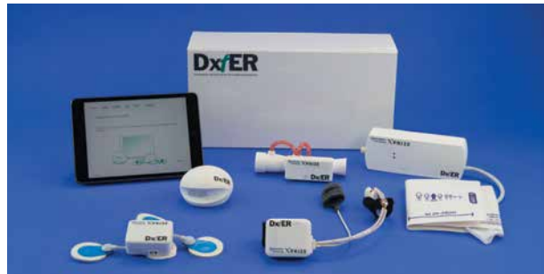
The prototype DxtER kit included an iPad Mini running a sophisticated diagnostic engine and a collection of noninvasive sensors.
