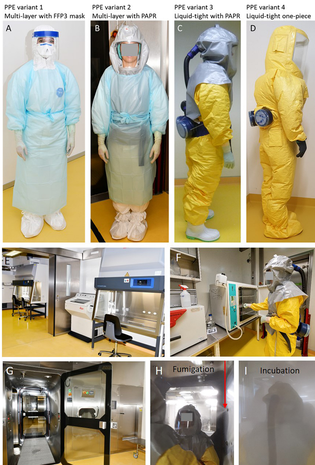
FIGURE 1 | (A) Personal protective equipment (PPE) variant 1 consists of a single-use coverall (Cat. III, type 4-B/5-B/6-B), apron with long sleeves, a double layer of shoe covers worn over crocs, a double layer of differently colored gloves, e.g., green nitrile gloves as the inner layer and white gloves as the outer layer, FFP3 mask, goggles and face shield. (B) PPE variant 2 corresponds with variant 1 but FFP3 mask, goggles and face shield are replaced by a powered air-purifying respirator (PAPR, e.g., Jupiter™ Air Filter Unit with two A2BEKP filters and 8 h rechargeable batteries) connected to a hood assembly providing head, face and shoulder coverage. (C) PPE variant 3 consists of a Tychem 2000C protective suit (Cat. III, Type 3/4/5/6) which protects against biological substances, and is impermeable to liquid and particles. Outer layers of gloves and chemical protective boots are sealed with adhesive tape. The hood is ventilated by the same PAPR used in variant 2. (D) PPE variant 4 consists of a one-piece Tychem ProChem protective suit (CPM F1 H L2, Cat. III, Type 3/5) with integrated boot socks and gloves, resistant against (Continued)
