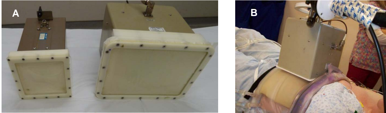
Figure 2 – FDA approved waveguide applicators available for superficial hyperthermia treatments in USA. A) MA-100 (left) and MA-120 (right) applicators with BSD rigid frame water coupling bolus (Pyrexar Medical - Salt Lake City UT); B) MA-120 applicator over custom conformal waterbolus which couples to widespread chestwall recurrent disease.
