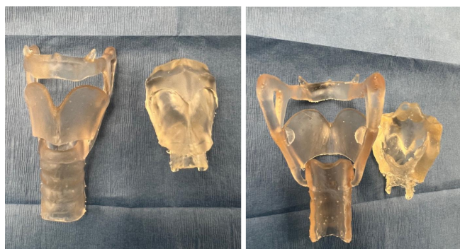
FIGURE 2 Anterior and posterior views of the 3D-printed, open-source, larynx model and endolarynx structures.
