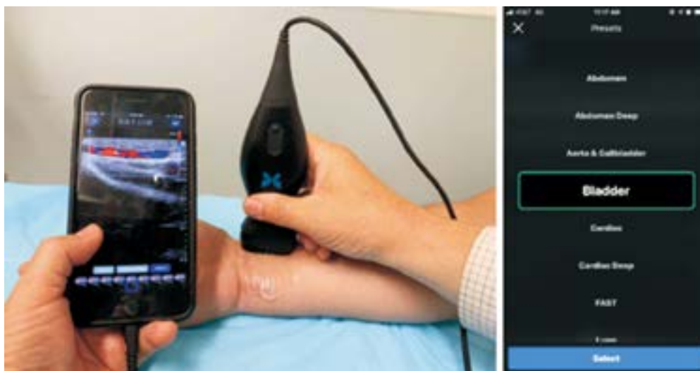
Figure 2 (A) A handheld Butterfly iQ unit is used to scan the radial artery; (B) There are 19 preset applications available for whole body examination and a few are shown here.
