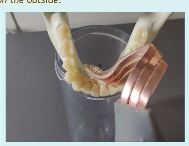
• Solution: Features a thin, flexible head that can be contoured to the back of teeth via tongue, and a telescoping handle for variability in arm positions.
