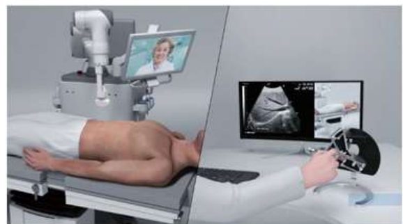
Figure 15 A robotic tele-ultrasound system (MGIUS-R3, MGI Tech Co., LTD., Shenzhen, China) can be used to remotely scan patients and communicate with doctors for diagnosis and consultation. Image provided by MGI Tech.
