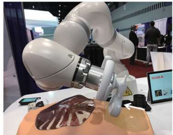
Figure 14 A light-weight six-axis robot system (Kuka, Augsburg, Germany) is depicted with the capability to maneuver and stabilize an ultrasound probe (arrow).
