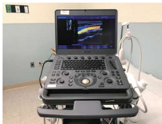
Figure 11 Narrow profile laptop-based ultrasound machines can facilitate portable ultrasound examinations (X5 model, SonoScape Medical Corp, Shenzhen, China).
