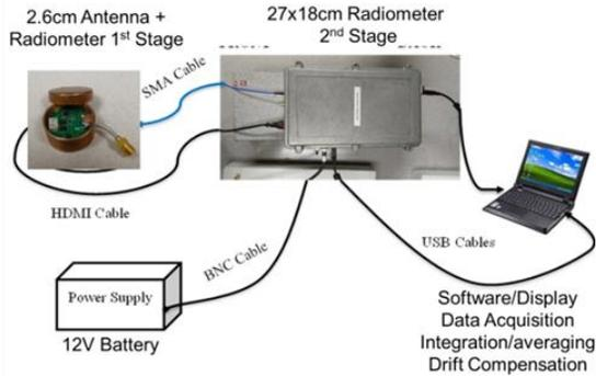
Fig. 1 Basic configuration of high-sensitivity microwave radiometry system.
