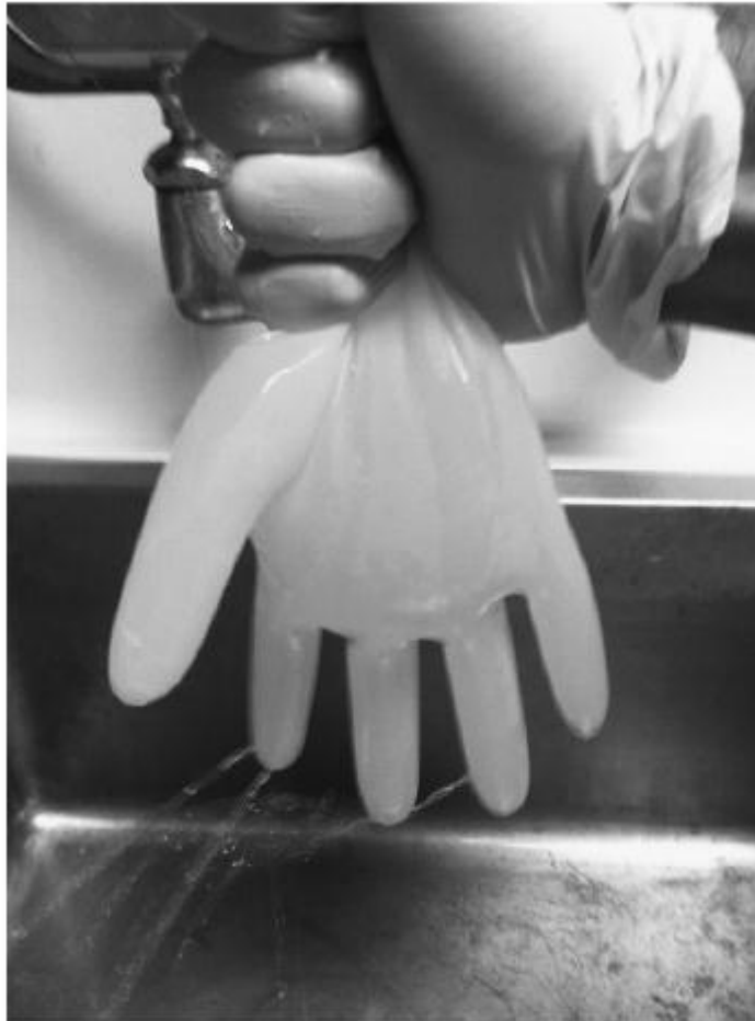
Fig. 1. Water infusion method for detection of glove perforations.
