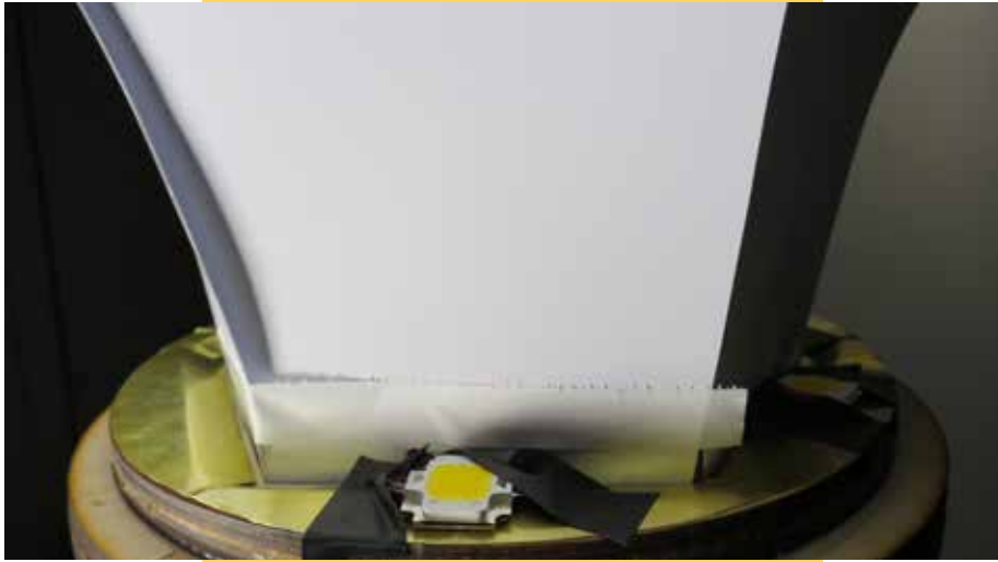
One of two high powered LED chips mounted to a brass plate to distribute the heat
