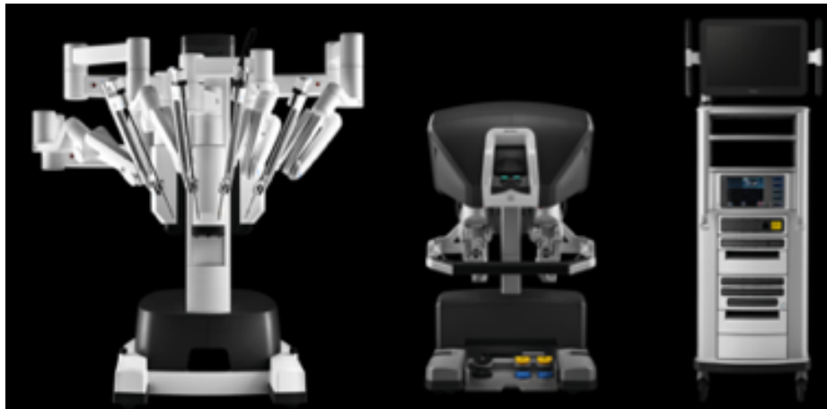
Figure 2. Da Vinci Xi Surgical System: patient cart, surgeon console, and vision cart. 9
