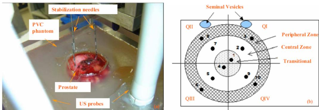
**Fig. 1:** Experimental setup (a) experimental platform; (b) distribution of needle insertions. The two ultrasound probes in the figure were used to capture the needle insertion procedure for post-evaluation, i.e. tissue deformation, needle bending, etc.
