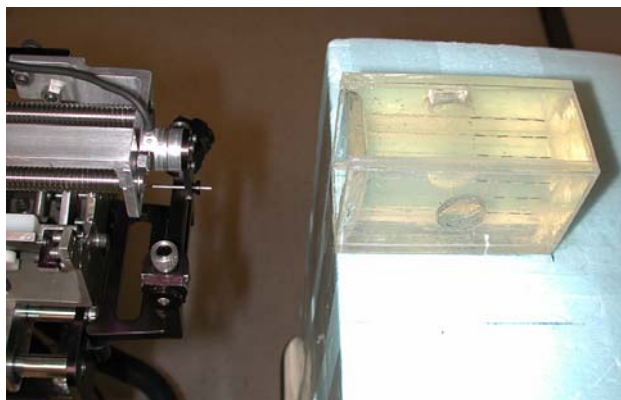
Figure 13: seed delivery in soft material (polyvinylchloride) phantom.
