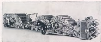
3-Cylinder Set of Woolen Cards with Broad Band Feed and Tape Condenser
