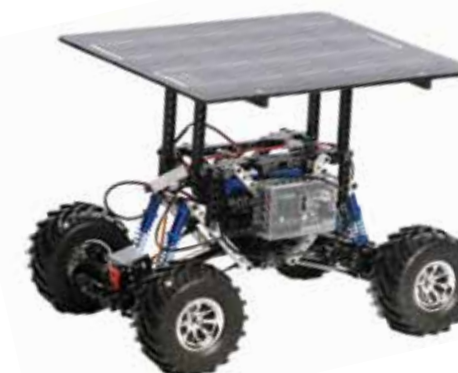
Kander is pictured with a solar-powered rover — built by PhilaU engineering faculty and students to research and test alternative power sources. Students in the mechatronics course this spring researched the use and functionalities of a solar-powered vehicle where solar energy was converted and stored in a lithium battery.
