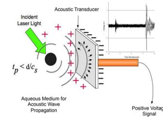
Fig. 1 - Schematic of photoacoustic method highlighting thermoelastic expansion of chromophore and signal transduction.
