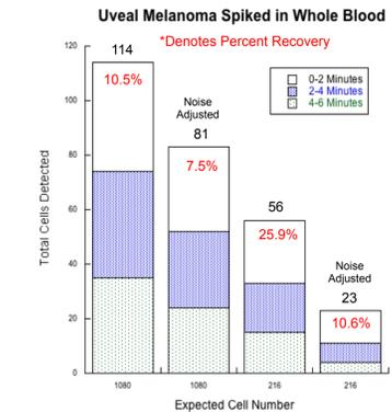
Fig. 7 - Various concentrations of UM002B cells spiked into healthy whole blood, isolated for PBMCs and analyzed. Expected cell number adjusted for 60% CUMC loss during isolation. **Ability to detect 1 CUMC in 10** present in noise adjusted whole blood sample.
