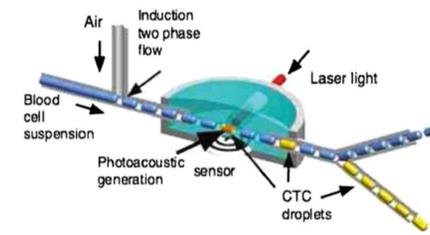
Fig. 2 - The photoacoustic flowmeter separates continuous flow of blood cells and immiscible air bubbles. Droplets containing pigmented cells are isolated for further analysis while the negative droplets are diverted for disposal.
