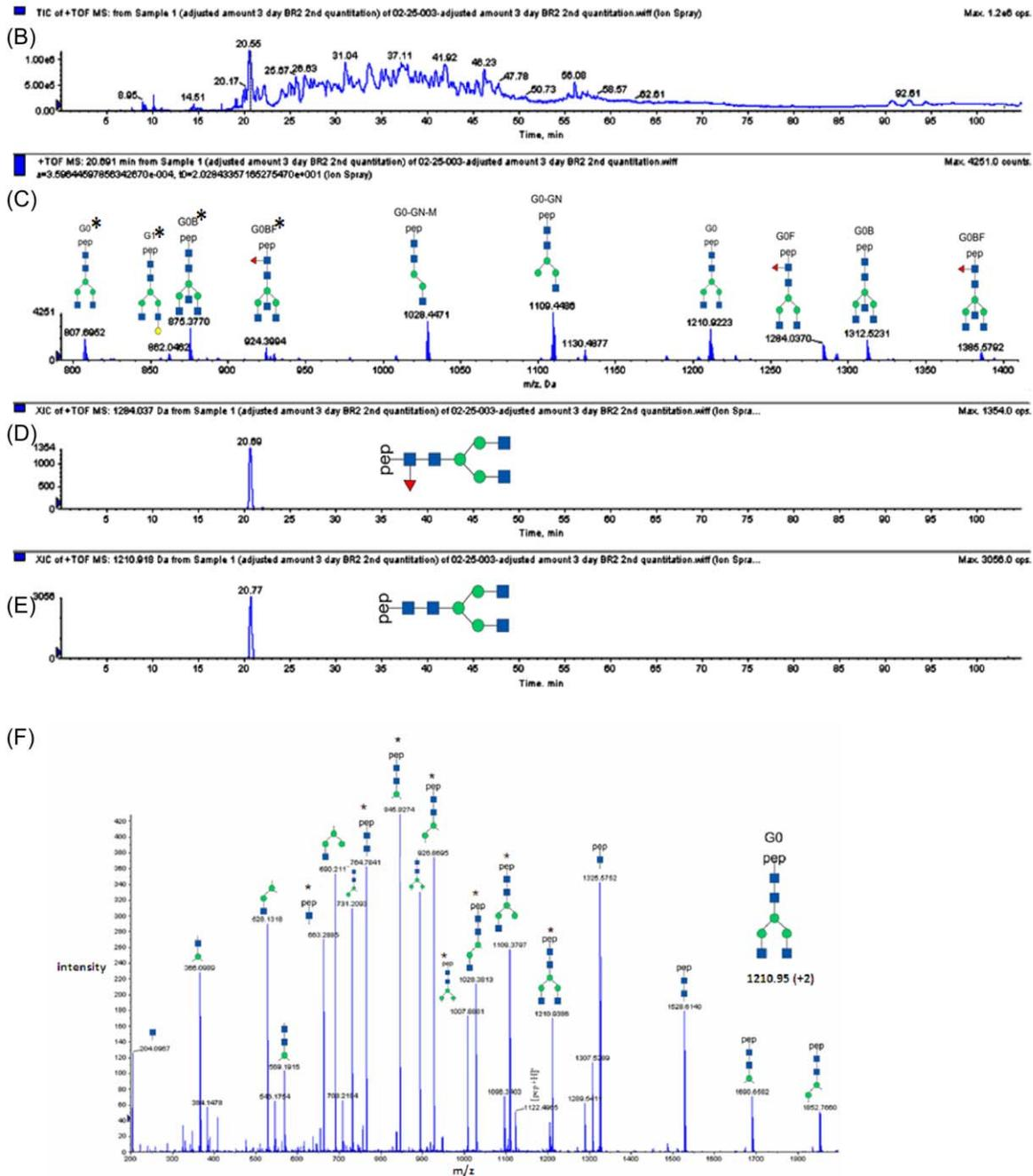
**Figure 5. Use mass spectrometric identification and glycoform profiling of the IgG glycoforms and AAL-reactive IgG.** (A) Scheme of the procedure (see details in Experiment and Methods Section); (B) A total ion chromatograph of a purified rabbit IgG; (C) A mass spectrum of the sample at retention time 19 minutes; (D) and (E) Extracted ion chromatographs of G0F, and G0, respectively. (F) MS/MS spectrum of G0 IgG. doi:10.1371/journal.pone.0044422.g005
