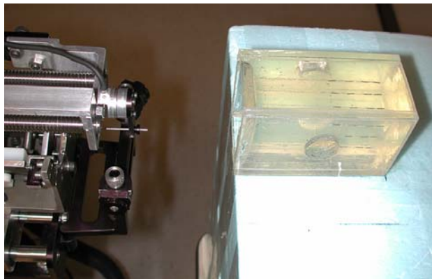
Figure 13: seed delivery in soft material (polyvinylchloride) phantom.
